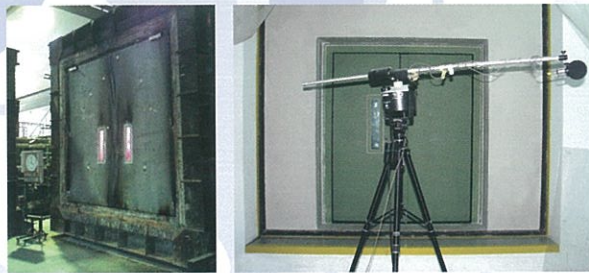
ABOVE: SIAC factory in Kuala Lumpur, Malaysia BELOW L: Fire-tested door at PSB for up to 4 hours BELOW R: Acoustic Door Test
